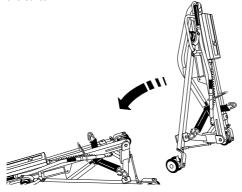
**2.** Place the folded Stowaway flat on the floor, resting on the rear castors and the folded boom. Engage the brakes on the rear castors.
