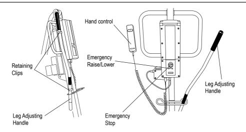
7. Remove leg adjusting handle from the storage clips on the mast and fit to the leg adjusting lever through the gate on the mast. Fit the battery pack to the mounting point on the mast and connect the power/charging plug to the battery pack.
