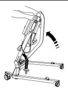
4. Swing the mast and boom upright and allow the mast to drop into the mast box.
