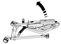
3. Stand facing the front castors and swing the leg retaining latches clear of the square handle on the mast. Move the legs sideways and downwards to place the front castors on the floor.
